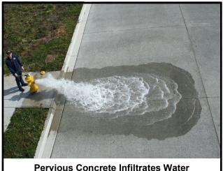
Pervious concrete can also reduce the impact of
